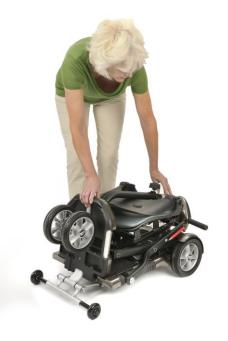
Once folded you can then lift your Minimo using the handle at the rear and stand it on its front wheels to move around in the folded position.
