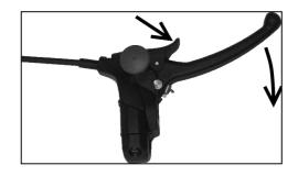
For unlocking the parking brake pull the brake handle backwards and unplug the red button.
