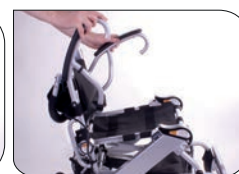
3 Fold backrest down then pull both arm rests anticlock-wise toward the back.
